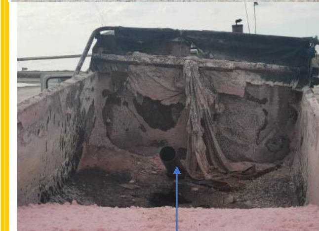
Broken Tipping cylinder through truck bucket
