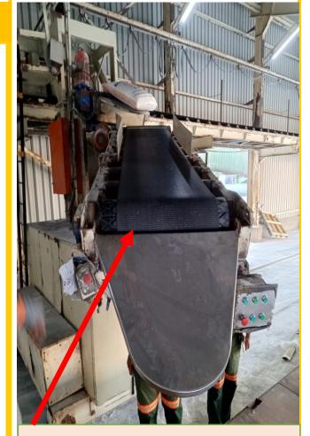
The gap between the conveyor pulley and the discharge plate.
